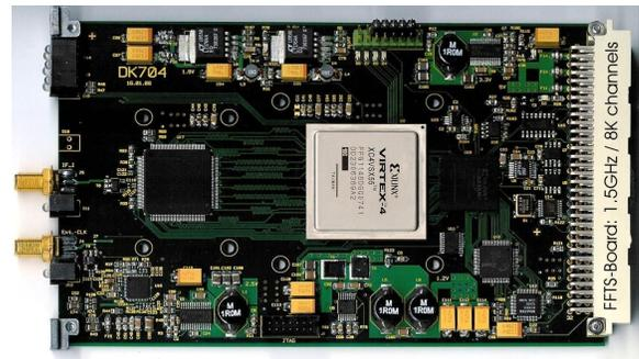
The MPIfR Array-FFTS, now operated at APEX, is equipped with 8 FFTS boards and the FFTS controller. A single FFTS board provides 1.5 GHz instantaneous bandwidth with 8192 spectral channels. The frequency resolution (equivalent noise bandwidth) in this standard configuration is 212 kHz.
