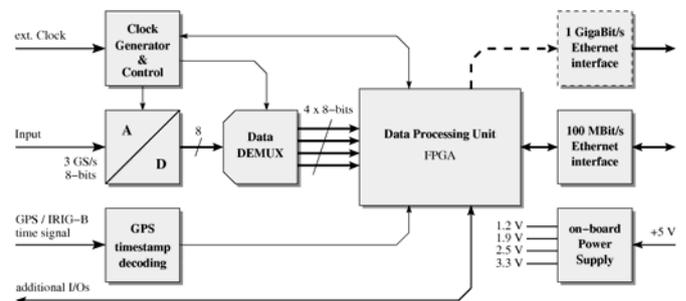
Fig. 2 Block diagram of the new MPIfR 1.5 GHz digitizer/analyzer board. The board can be equipped with a single- or dual-input ADC (ADC083000 or ADC08D1500). The optional GigaBit Ethernet interface allows high speed data acquisition with transfer rates up to 85 MBytes/s, which are required for pulsar or transient searches.
